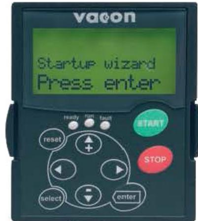
*Frequency converter display and keypad push buttons (inside control box +OP6).*
